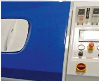
Cyclic corrosion chamber
