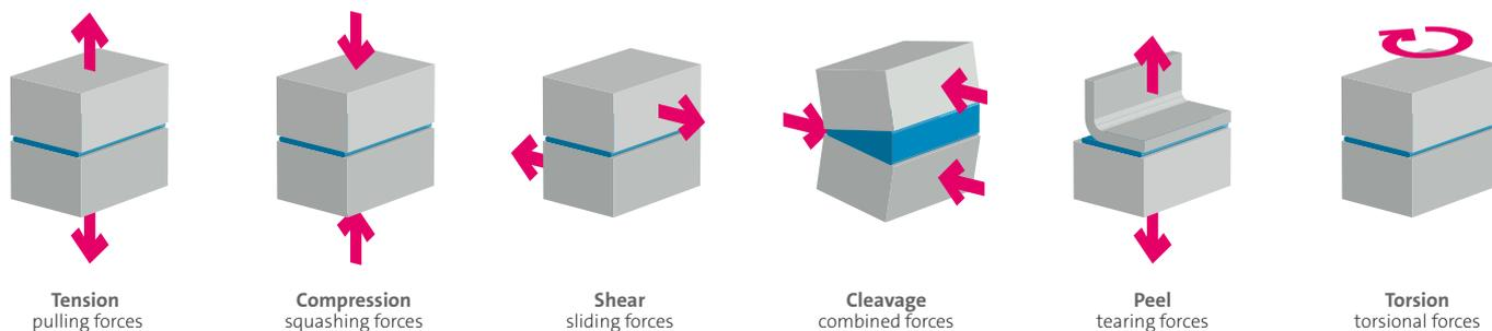
Strong bonded joints need to be designed that the loading stresses will be directed along the lines of the adhesive's greatest strengths. A poorly designed joint can lead to high-stress concentrations in the joint itself and/or in the substrates connected. Adhesives are more resilient under shear, compression and tension stresses. Cleavage and peel loading are the most severe as they concentrate the applied force into a single line of high stress.
