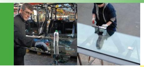
Far left: Used as part of a complete direct glazing system, BETAPRIME is also used as an adhesion promoter on body surfaces in conjunction with BETAMATE<sup>™</sup> structural adhesives.
