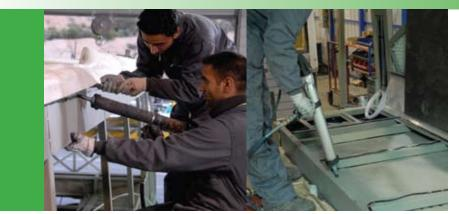
Far left: BETAMATE structural adhesives reduce vibration by stiffening overall vehicle structure.
