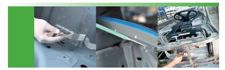
Advanced materials technologies enable Dow Automotive Systems to provide a wide range of seam sealant and adhesive solutions based on specific customer requirements. Sealing vehicle body joints and seams provides added protection against corrosion while also protecting interior compartments from dust, dirt and moisture. Sealants from Dow Automotive Systems also achieve bonding, acoustical and thermal improvements in commercial vehicle applications.
