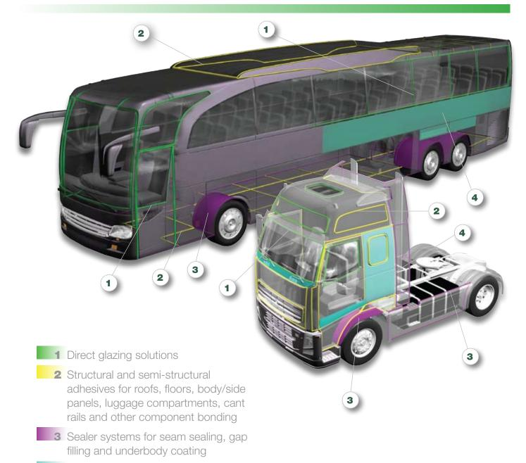
4 Acoustical/structural foams that provide acoustical or energy management properties
