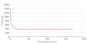
ASTM D1876 — Aluminum — 0.3mm bond gap — 10mm/min
