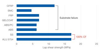
STM D1002 - Metals - 0.3mm bond gap - Plastics - 1mm bond gap - 10 mm/min
