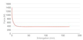
ASTM D1876 — Aluminum — 0.3mm bond gap — 10mm/min
