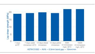
\* 4 hours at -30°C + 4 hours at 80°C + 16 hours at 30°C/80%RH. Repeated 8 times. Cohesive failure is at 100%.
