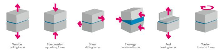
Strong bonded joints need to be designed that the loading stresses will be directed along the lines of the adhesive's greatest strengths. A poorly designed joint can lead to high-stress concentrations in the joint itself and/or in the substrates connected. Adhesives are more resilient under shear, compression and tension stresses. Cleavage and peel loading are the most severe as they concentrate the applied force into a single line of high stress.
