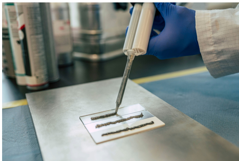
Adhesive tests in a laboratory help when choosing an adhesive. © Bodo Möller Chemie GmbH
