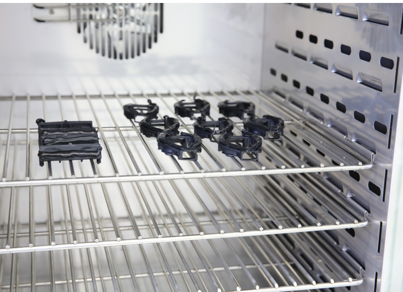
Aging tests are used to simulate how the bond behaves under high stress loads over time. © Bodo Möller Chemie GmbH
