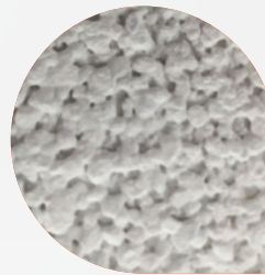
Figure 1. Without PlastGard® – Pinholing
