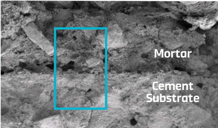
SEM image of the interface of a mortar-cement substrate after subjected to the tensile strength test.
