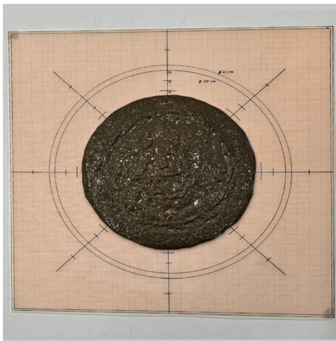
Effect of TARGON® FM (0.2%) in self leveling floor screed: spreading diameter after 30 sec: ~15 mm vs 8 mm without.
