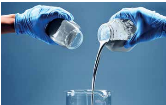
Left: Pigment preparation without dispersing agent. Right: Pigment preparation with 0.1% POLYRON® N. Adding just 0.1% POLYRON® N, the viscosity can be strongly reduced at the same PVC, thus a flowable paint can be achieved.
