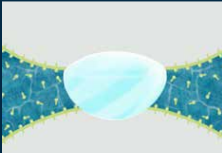
Figure 1 (Bridging Mechanism): Defoamer drop breaks through the foam lamella on both sides.
