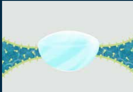
Figure 2: Dewetting of the defoamer drop.
