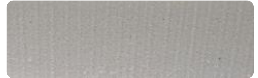
Lightweight closed cell structure with 0,55-0,6 kg/L density
