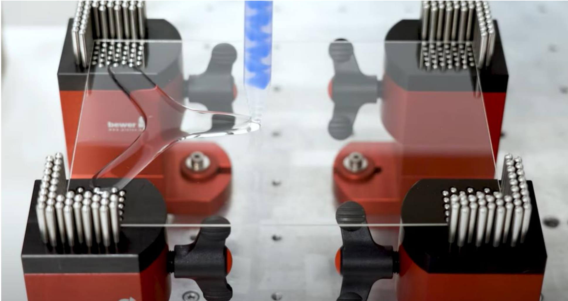
Display Production: Optical Bonding with 2-Component Material WACKER SilGel613 (youtube.com)
