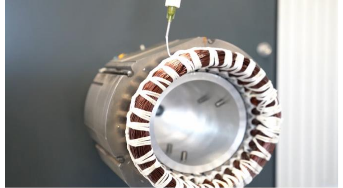
ViscoTec Trickling System: Resin Impregnation of Rotor & Stator with Dolphon 1180 HTC from von Roll - YouTube
